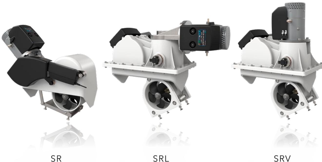
For boats that cannot fit a tunnel thruster or do not wish to have an external thruster under the boat, then a retractable thruster is the solution. Side-Power have designed a product range that is focused on practical sturdiness, uncompromised safety and quick deployment.
